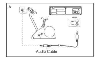
B. Plug one end of a 1/8" to RCA stereo audio cable (available at electronics stores) into the jack beneath the console. Plug the other end of the cable into an RCA Y-adapter (available at electronics stores). Next, remove the wire that is currently plugged into the AUDIO OUT jack on your VCR and plug the wire into the unused side of the Yadapter. Plug the Y-adapter into the AUDIO OUT jack on your VCR.
